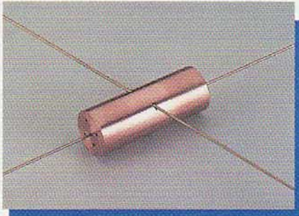
■ Drilling flushing holes in copper electrode.
