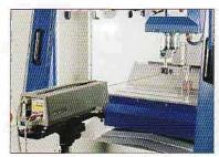
All 3 axes are checked by a laser inspection system to ensure positioning accuracy and repeatability.
