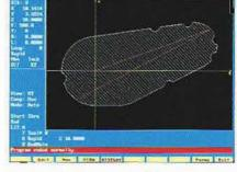
Using the conversational programming language, the full compliment of canned cycles and the integrated geometric calculator, complex parts can be programmed easily on the VMC.
