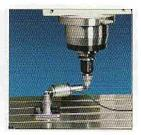
A "state-of-the-art ball bar test" confirms squareness and accuracy of micro movement.
