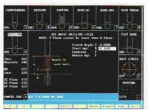
Basic drilling canned cycle example....
