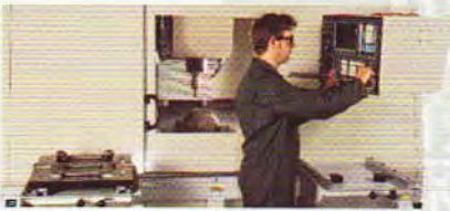
Machine in cutting cycle while second pallet is in position for reloading
